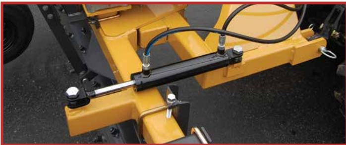
Angling capability powered by the tractor hydraulics
