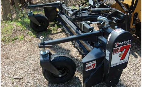
Harley comes with a standard toggle hydraulic control box. Can be ordered with an in-cab attachment controller harness.
