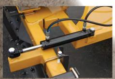
Angling capability powered by the tractor hydraulics
