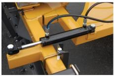
Angling capability powered by the tractor hydraulics
