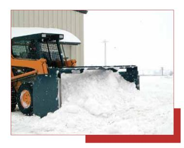
The FFC® Snow Push, by Paladin is engineered of heavyduty, fully welded steel with 3/8" thick end plates to capture and remove even the heaviest snow without leaving windrows or spillover. For SSL, Compact Utility Loaders, Small Wheel Loaders and Backhoe Loaders..
