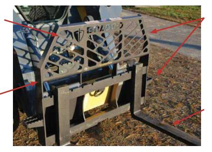
Angled side corners and step for easy and safe side access in and out of operator
