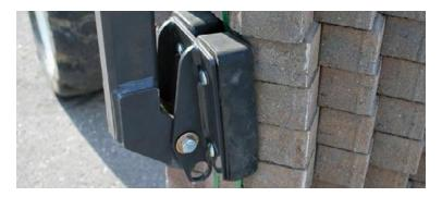
A cylinder check valve prevents loss of clamping force even if the machine's hydraulic power is lost
