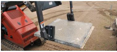
Automatically adjusts the position of the clamping arms to ensure a good grasp of the material
