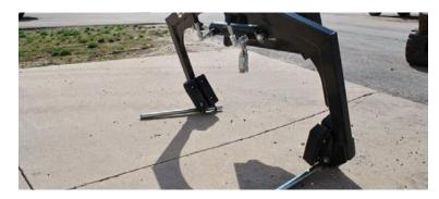
A simple stand utilizing two steel tubes has been integrated into the attachment that stores neatly into the quick attach assembly when not in use
