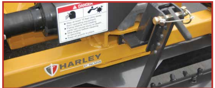
Each position change allows the effective surface of the roller to grow. Each position has a different effect on the material being prepared.
