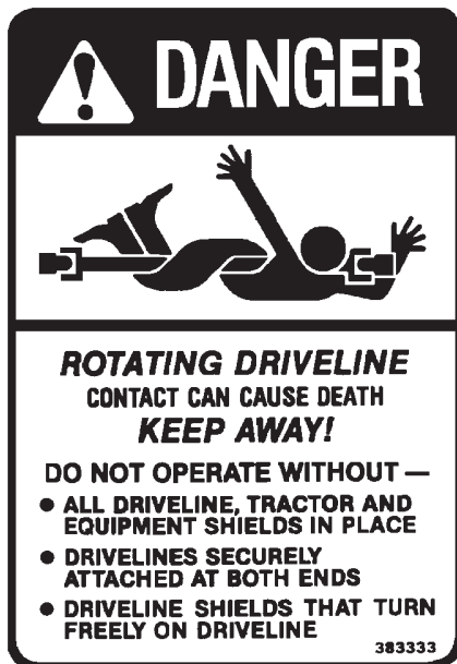
DANGER! ROTATING DRIVELINE PART #4286 (LOCATED ON PTO)
