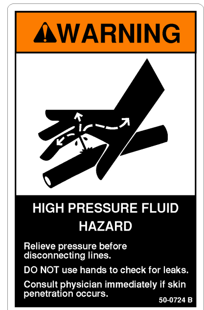
# 50-0724 WARNING! HIGH PRESSURE FLUID HAZARD
