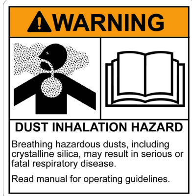
# 41043 WARNING! HAZARDOUS DUST
