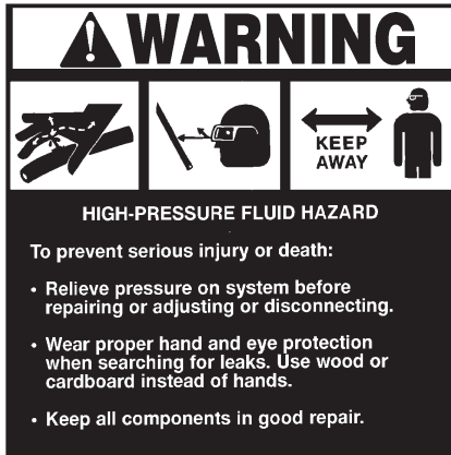
PART #40151 WARNING! HIGH PRESSURE FLUID
