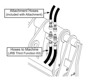
Typical arrangement shown. Actual coupler bulkhead arrangement will vary.
