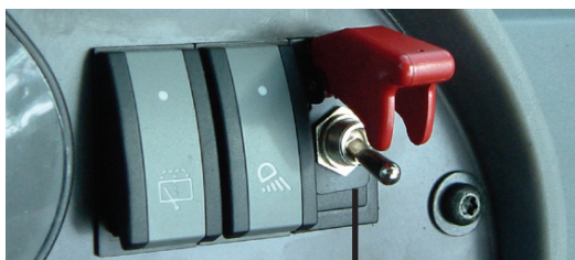
fig 3.24 Example of a Miller style on/off operating switch
