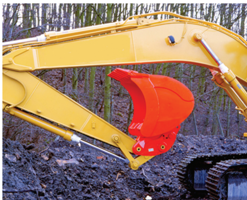
fig 2.4 Miller Scoop Bucket and Miller Coupler
