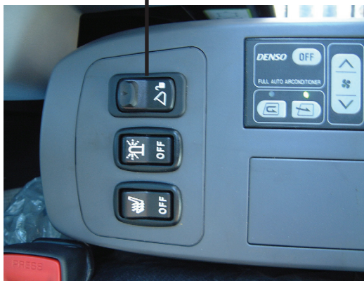
fig 3.23 Example of an OEM style on/off operating switch. (Switches differ with machine interior)
