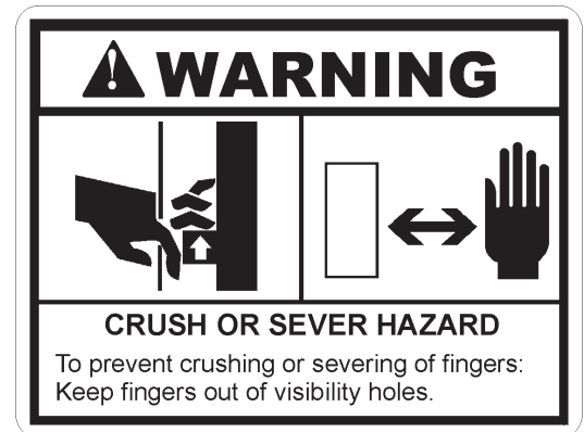
PART #41112 WARNING! CRUSH OR SEVER HAZARD
