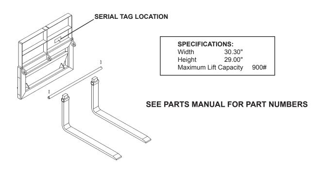
WARNING! DO NOT EXCEED THE LIFT CAPACITY OF EITHER THE LOADER OR THE TINES.
