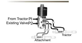
Used to convert existing tractor loader 2-function hydraulics to allow a 3rd function for controlling various hydraulic accessory attachments, for example hydraulic grapples and multipurpose buckets. Can plumb into existing loader bucket cylinder circuit.
