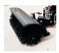
RMRM - Compact Tractor Angle Sweeper - Mechanical 3-Point Drive Features rear-mount mechanical drive driven from rear 540 PTO. Angles manually 30° left or right. Includes steel hood, chain shield, height adjustment chains, and mounting pins. T-Shaft gearbox allows for reversal of brush rotation of mechanical drive.
