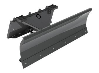
The **114 Series Snow Blade** is available in either hydraulic or manual angle. For Skid Steers, Compact Tool Carriers, and Compact Utility Loaders.
